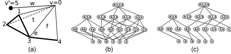
Figure 1: (a) A simplicial 3-complex, and the graph-based representation of the immediate (b) boundary relations  $\mathcal{R}_{p,p-1}$  and (c) partial co-boundary relations  $\mathcal{R}_{p,p+1}^*$  among its simplices, which are encoded in the *Incidence Simplicial (IS)* data structure [7]. We call them *mangroves*, and they are the basis of our *Mangrove Topological Data Structure (Mangrove TDS)* framework.
